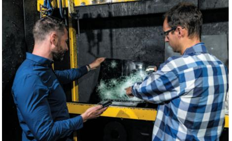
However, every time a new generation of a luxury car is released, it is a new challenge that starts from scratch. "Our official test for whether armoured glass can withstand the impact of .44 Magnum round is three shots in the form of a triangle, 120mm apart. If it passes, the glass is signed off as B4 specification. Obviously, we want to make doubly sure it is safe, so the glass can actually handle a higher calibre gun, however we will sign it
