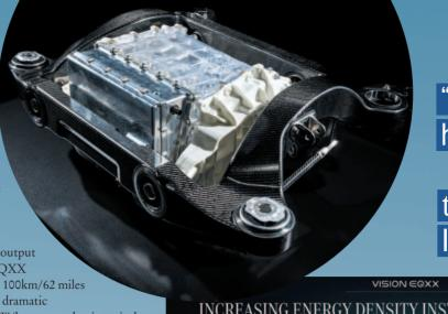
"This new battery is half the volume and 30 per cent lighter than a conventional lithium-ion battery"
